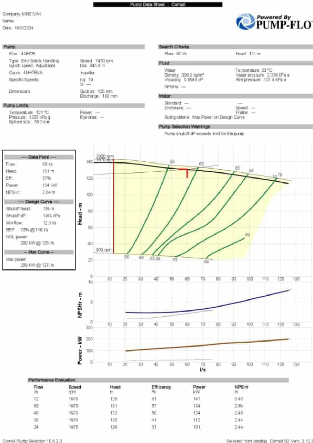
Figure 4-17: Normal Operation (Duty Point 1): The duty point is achieved with a 1x duty pump operating at a reduced speed of 1970 RPM, at a pump efficiency of ±57%.
