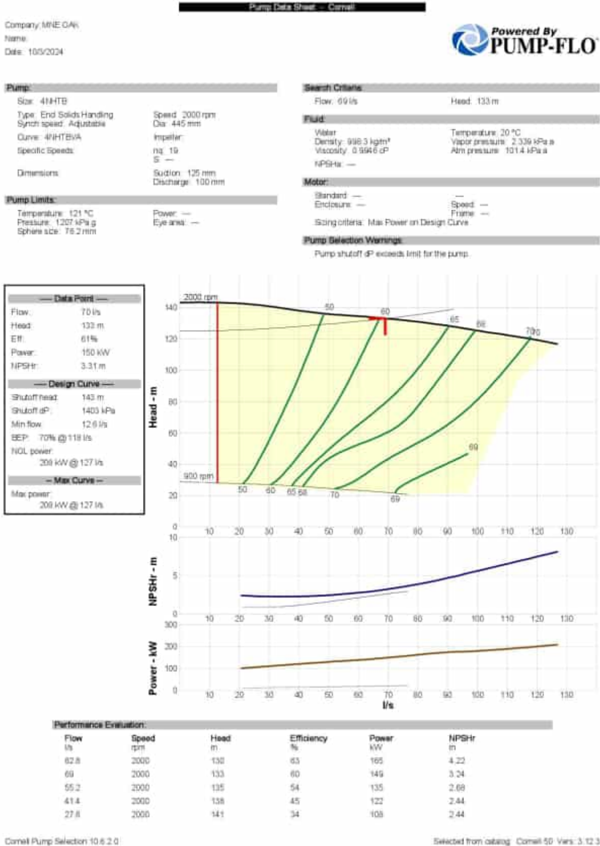
Figure 4-18: Extreme Events (Duty Point 2): The duty point is achieved with 1x pumps operating in parallel at 2000 RPM, at a pump efficiency of ±60%.
