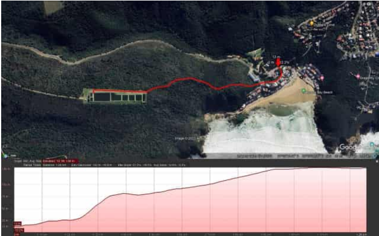
Figure 4-32 Pipeline route and vertical profiles for the pipeline between PS4 to WWTW
