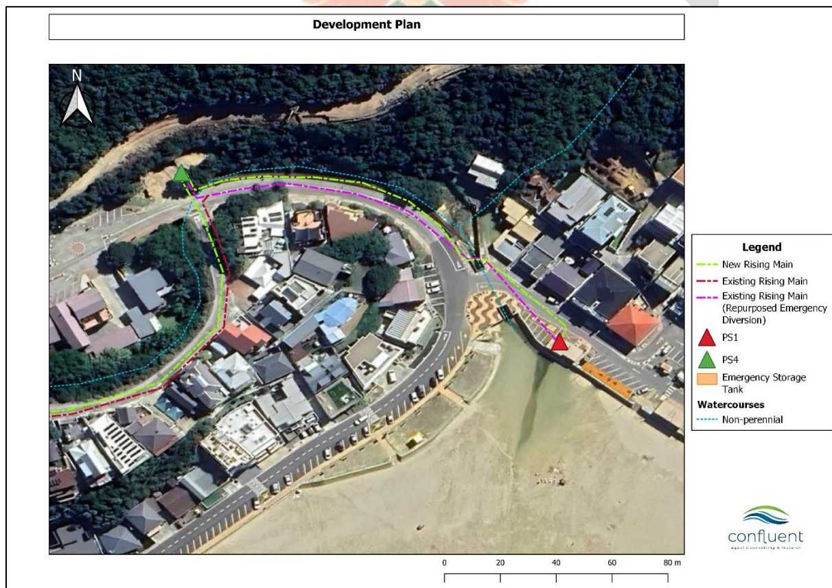
Figure 4: Map indicating configuring of pipelines between PS1 and PS4
