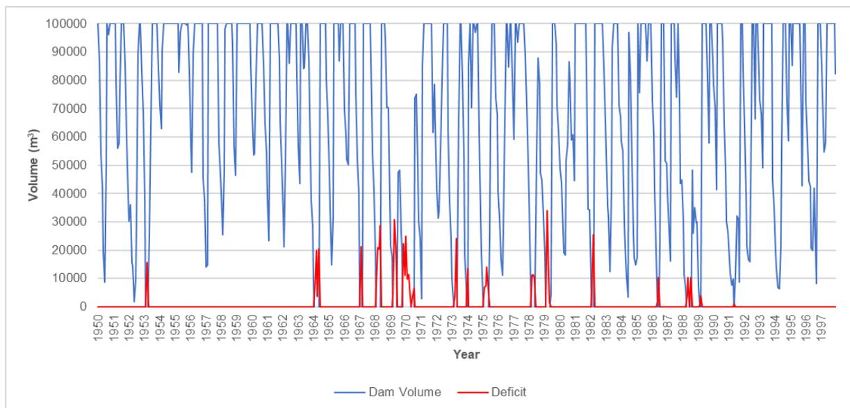
Figure 9: 50-year simulation with a 100 000  $m^3$  dam
