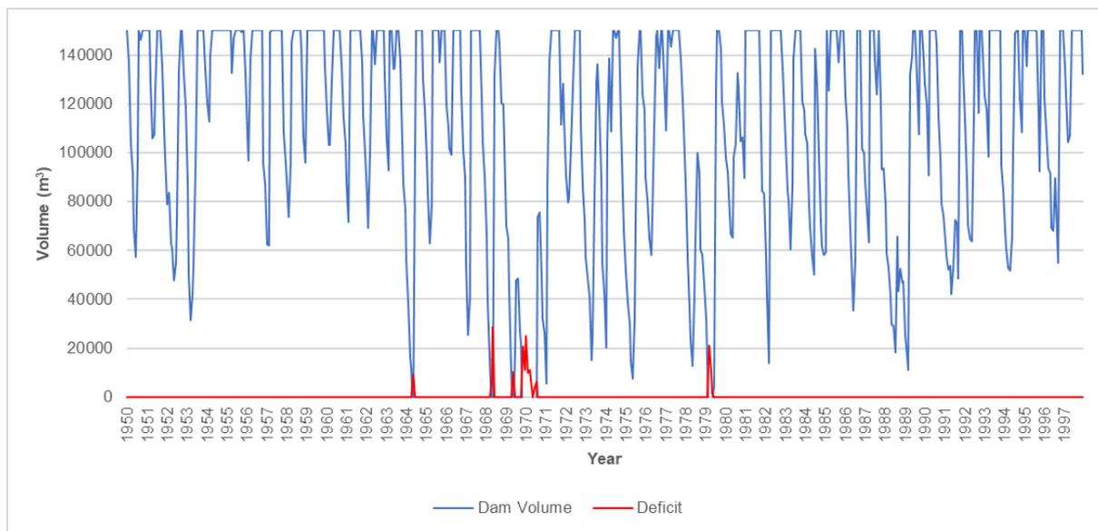
Figure 10: 50-year simulation with a 150 000 m<sup>3</sup> dam.
