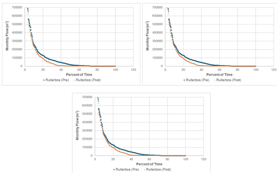
Figure 12: Flow duration curves illustrating the effect of different dam sizes on flow in the Ruiterbos River below the proposed dam.
