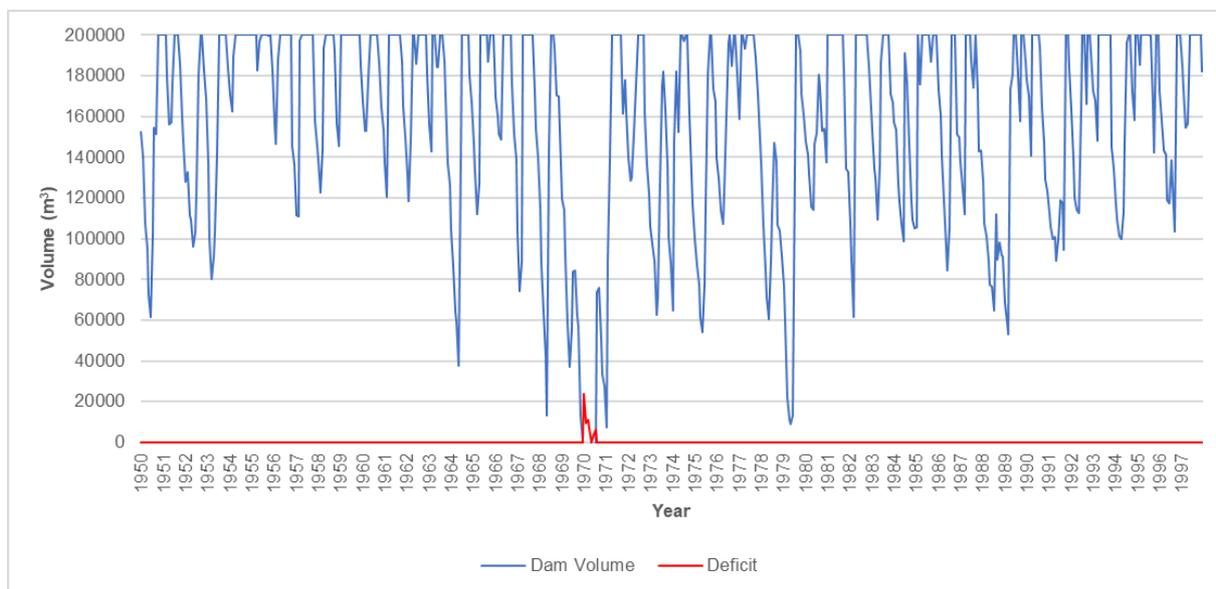
Figure 11: 50-year simulation with a 200 000 m<sup>3</sup> dam.
