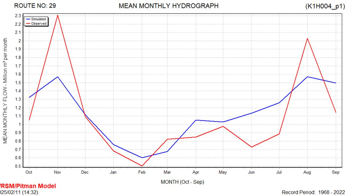
Figure 7: Mean monthly hydrograph for DWS flow gauge station K1H004.
