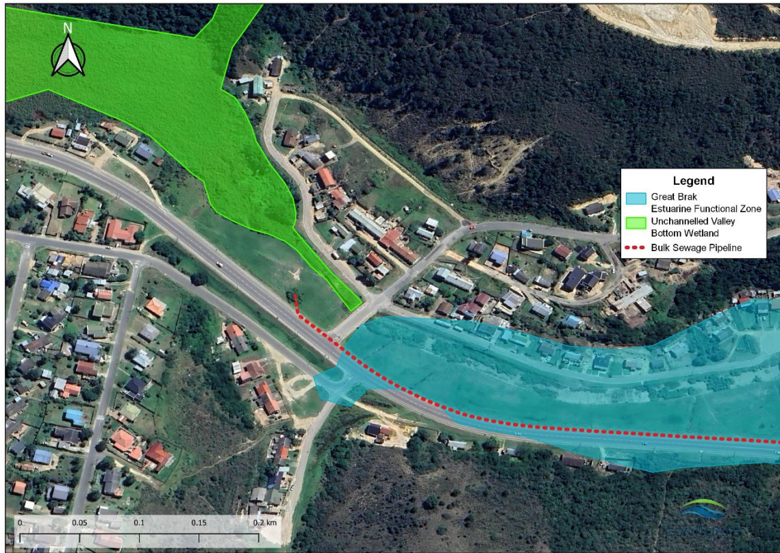
Figure 3: Map indicating the upper section of the bulk sewage pipeline upgrade that lies adjacent to an unchannelled valley-bottom wetland.
